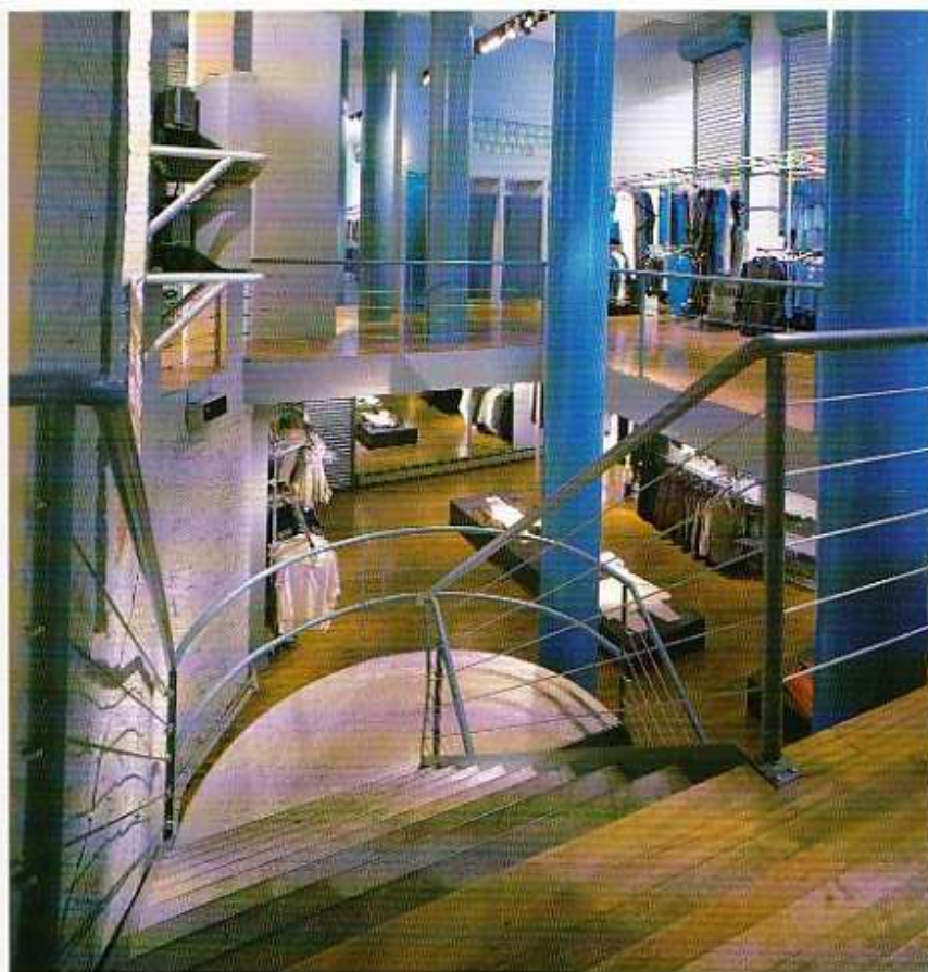
The original design of Paronon, New York, by Harry Farnow, shows how, for advanced store design from Tokyo and Paris to London, the design initially used a variety of basic materials. Rough concrete slabs and plaster walls provided a foil for the smooth maple wood floors, while the cast-iron columns were part of the original cast-iron construction of the building in the Union Square district. In 1996 this was redesigned with paneled concrete floors and concrete display platforms but nevertheless retaining the original character. (Photo: © Paul Wachtel 1994)
